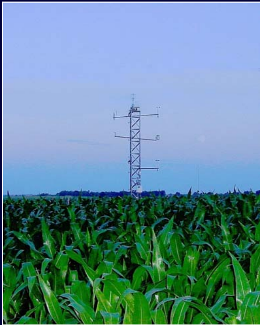
Landscape-level (Eddy Covariance) Measurement of CO 2 and Other Fluxes
