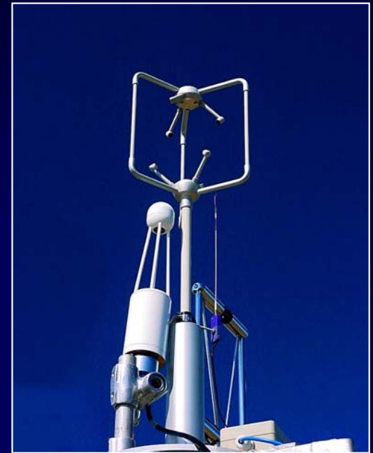
Close Up of Eddy Covariance Flux Sensors
