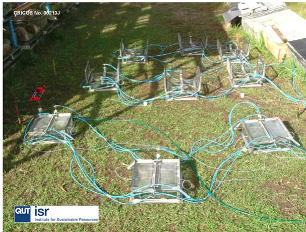
Automated chamber system used in Australia
