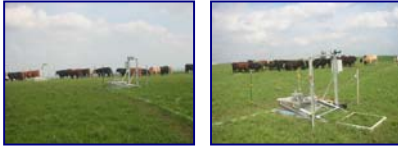
Fig. 1. A hot-wire system was used to protect the chambers while allowing the cattle to graze in the sample plot. Measurements of intercepted photosynthetically active radiation as well as routine visual inspections indicated no difference between the vegetation inside and outside the plot area. Clipped leaves were observed inside the plots, indicating that the cattle successfully grazed in the area encompassed by the soil frame despite the presence of the chamber system.
